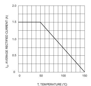
Fig. 1 Forward Current Derating Curve
