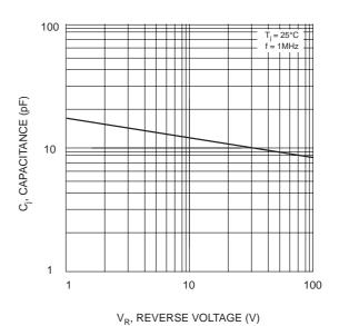
Fig. 4 Typical Junction Capacitance
